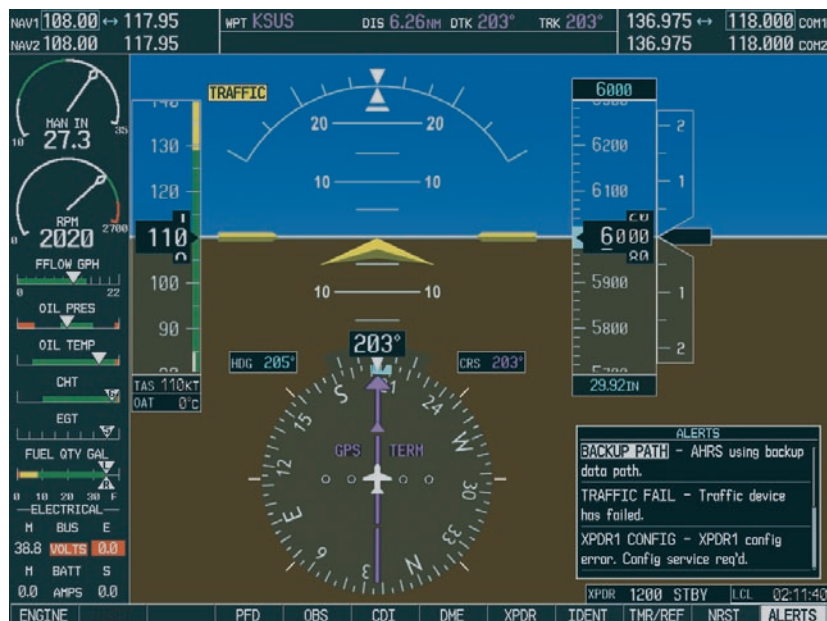
Figure 3.7.1 PFD Reversionary Mode
