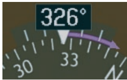
Figure 3.4.18 Turn Rate Indicator and Trend Vector
